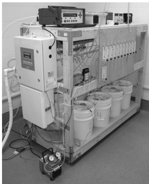
Figure 1. Emission vessel system used to evaluate the efficacy of various manure treatment agents to decrease ammonia emissions from manure storage.
