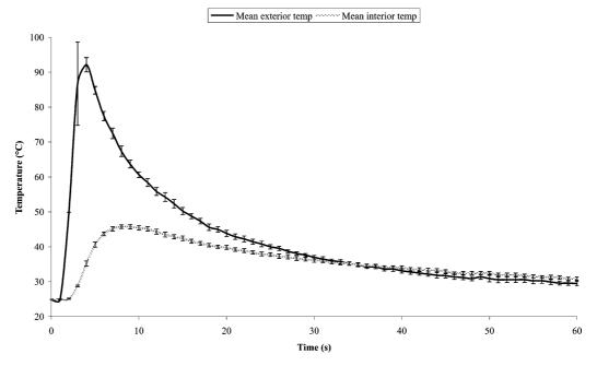
Fig. 4. Temperature plots of mean (n = 5) exterior and interior temperatures on the shells of eggs subjected to steam (100 °C) for 2 s.
