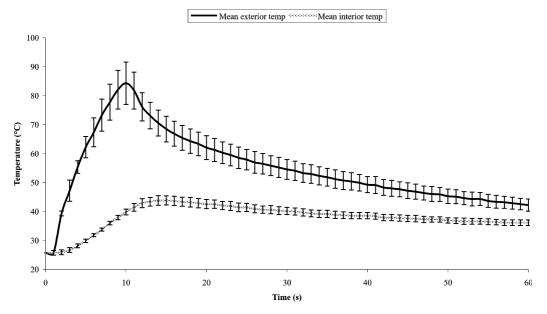
Fig. 1. Temperature plots of mean (n = 5) exterior and interior temperatures on the shells of eggs subjected to hot air (180 °C) for 8 s.
